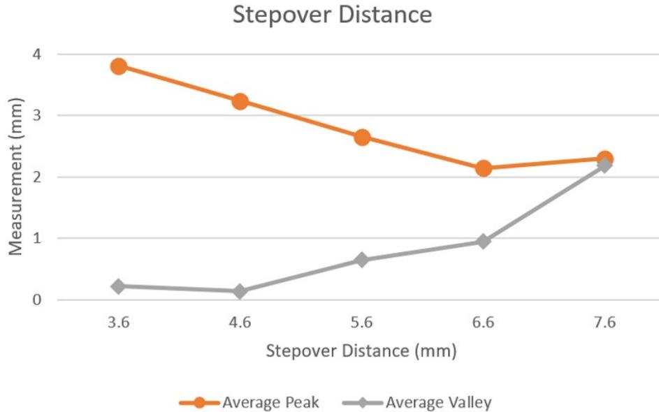
**Figure 9.** Average peak height and valley depth resulting from different step over distances.
