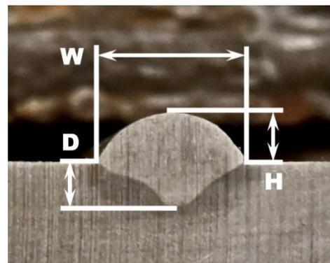
**Figure 4.** Weld bead cross section showing width (W), height (H), and penetration depth (D).
