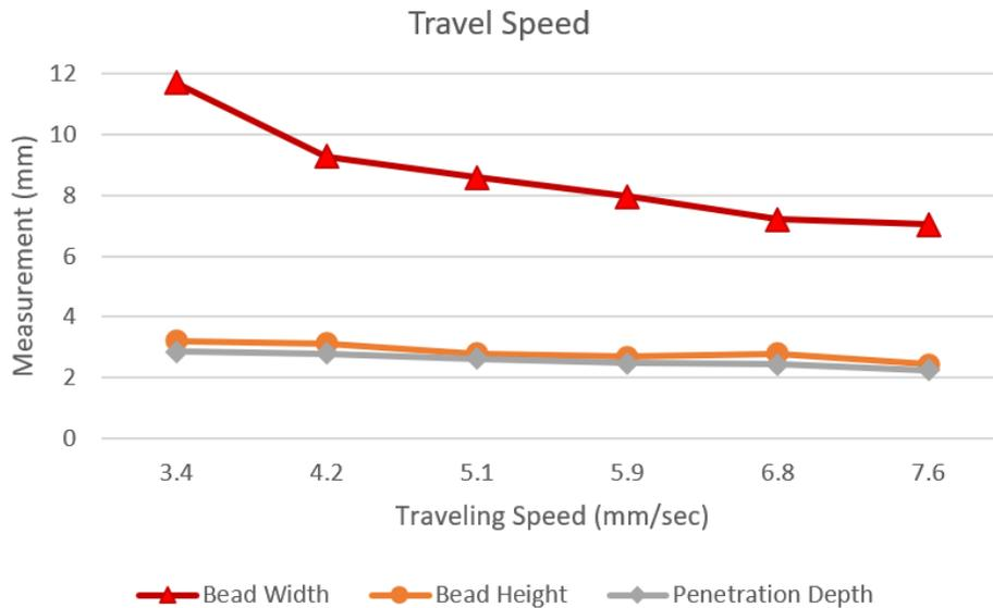
**Figure 6.** Relationship between weld geometry and the welding travel speed.
