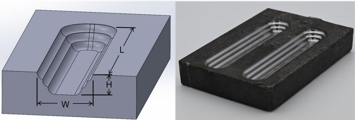
**Figure 3.** Terraced cavity geometry created using a bullnose endmill.
