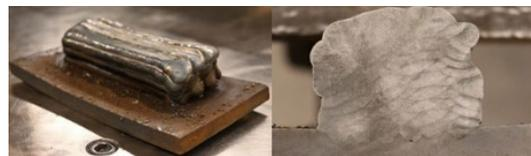
**Figure 8.** Demonstration 3D geometry from stacked layers with a 4.6mm step over.
