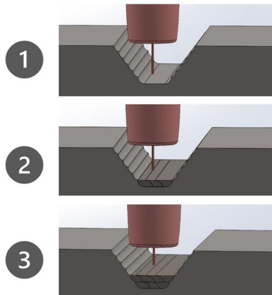
**Figure 2.** Cavity geometry and the weld filling strategy.
