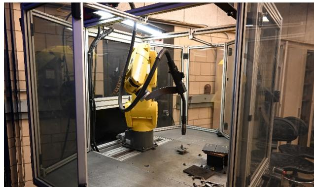
**Figure 1.** ArcMate 50iC industrial robot used for wire arc additive manufacturing of castings.
