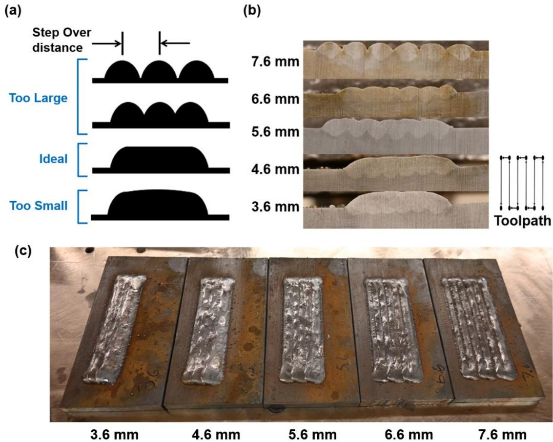
**Figure 7.** Geometry obtained by adjusting the step over distance with a travel speed of 6.8mm/s.
