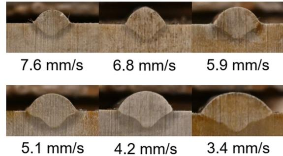
**Figure 5.** Etched cross sections of weld beads for each travel speed.
