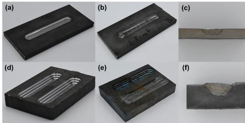
**Figure 10.** Production welding demonstration showing, a) single layer cavity, b) single layer weld, c) etched cross section of single layer weld, d) three layer cavity, e) three layer weld, f) etched cross section of three layer weld.
