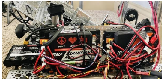
b. Hub and battery on the side of the robot
