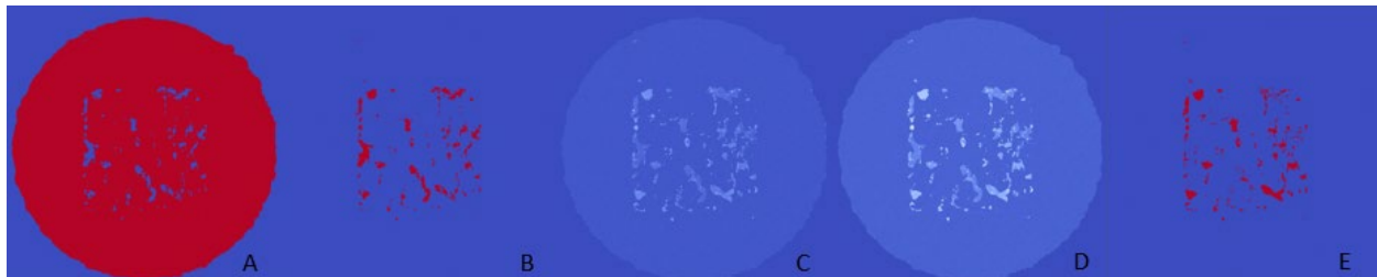
Figure 5 Binary Otsu classification of SEM TLD BSE 0° SEM Image: Otsu's method applied to the SEM image (a and b), Gradient Magnitude Fillhole (c), Median Gradient Magnitude Fillhole (d), Otsu's method applied to the Median Gradient Magnitude Fillhole (e)
