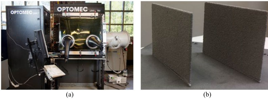
Figure 3. (a) The advanced imaging system installed in the OPTOMECH LENS 750 machine, and (b) final thin wall builds using Ti-6Al-4V material [5].
