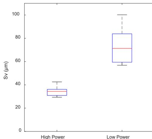
Figure 5: Comparison of  $S_v$  values for both high power and low power specimens, using the data from each of the twelve regions on the specimens.
