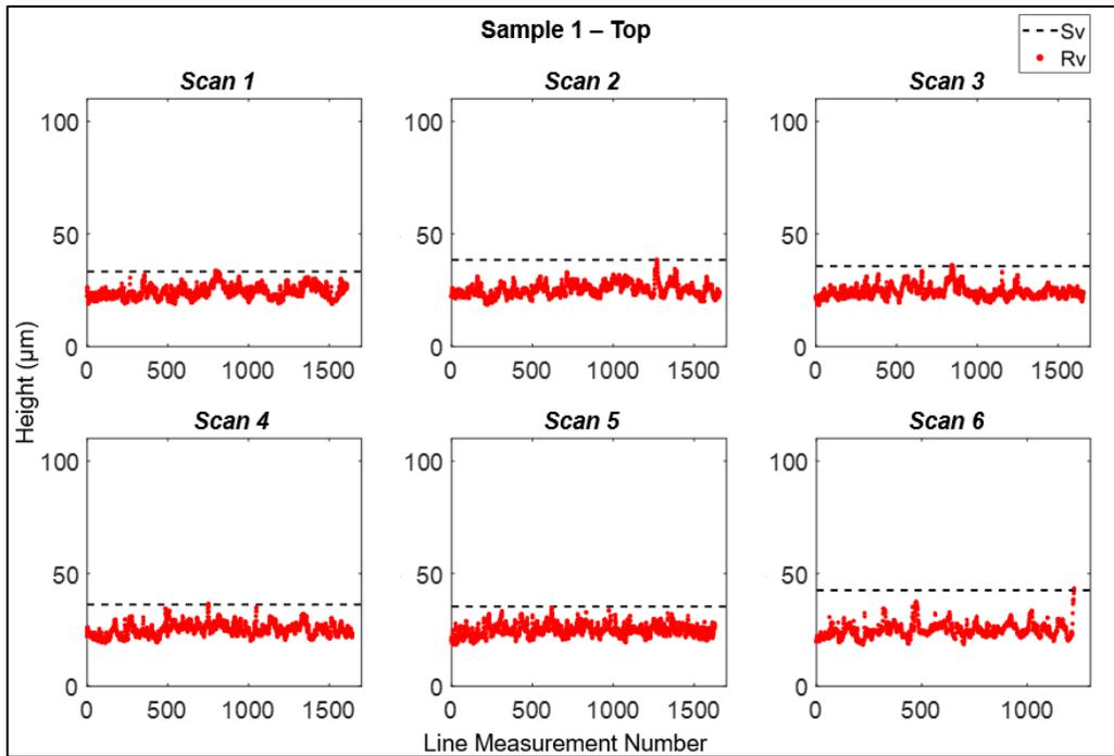
Figure 7: Rv and Sv measurements across the top of Sample 1.
