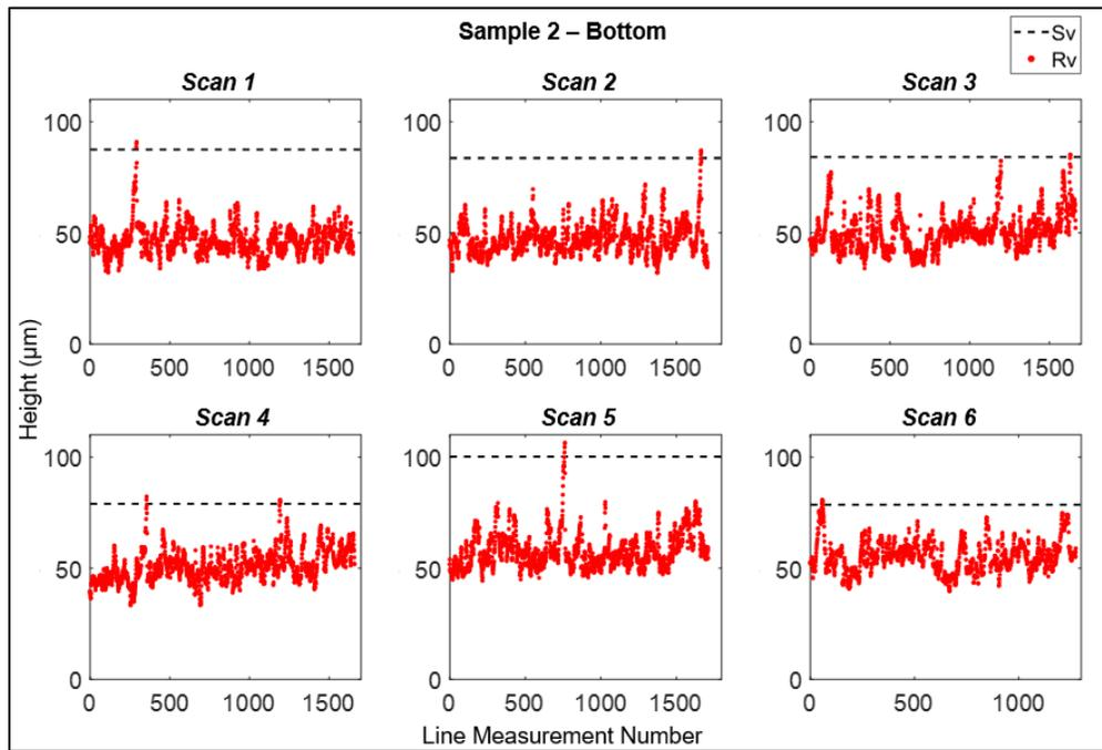
Figure 10: Rv and Sv measurements across the bottom of Sample 2.
