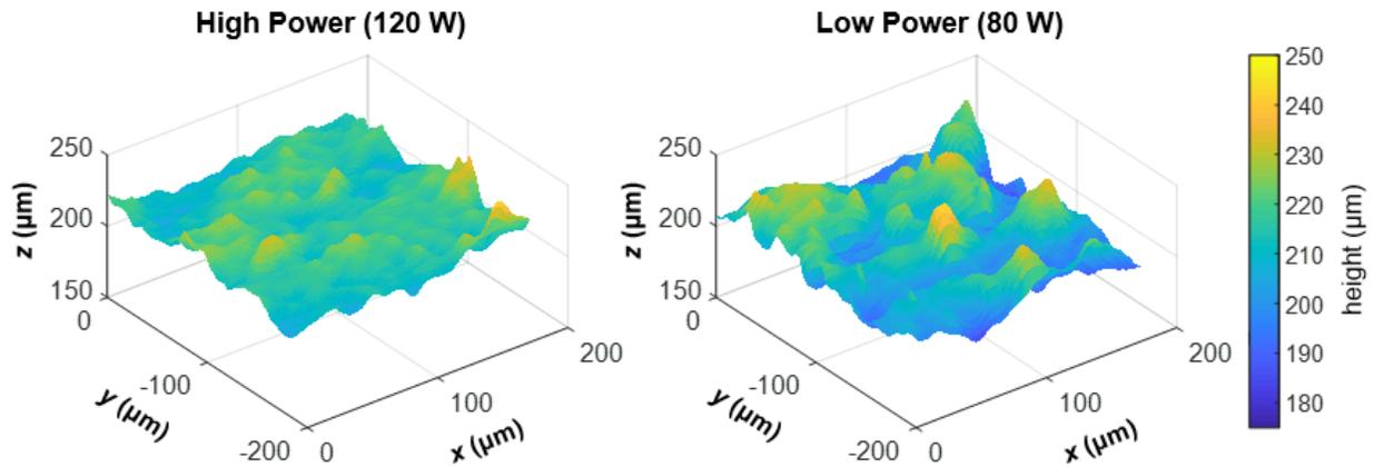
Figure 2: Sample surface roughness of both low power and high power AM surfaces.
