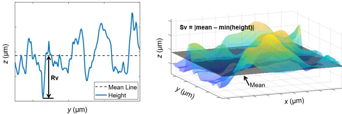
Figure 4: Comparison of  $R_v$  (left) and  $S_v$  (right) surface metrics.
