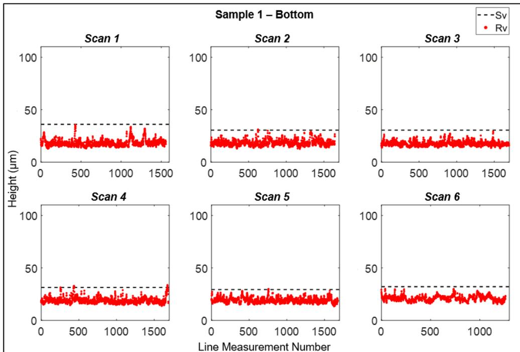
Figure 8: Rv and Sv measurements across the bottom of Sample 1.
