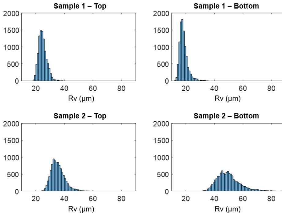
Figure 6: Histograms showing the variation of Rv within each of the samples.
