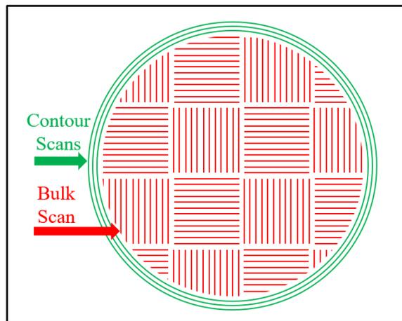
Figure 1: Contour scan versus bulk scan path in AM.
