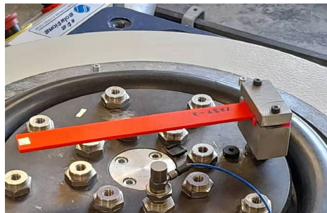
Figure 2 Boundary condition of modal analysis. Clamped-Free
