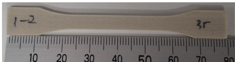
Figure 4. Specimen manufactured in powder bed temperature at 170 °C and layer thickness 0.05mm, energy per unit area of 0.175 J/mm 2
