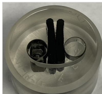
Figure 4, Two adjacent BAAM Samples mounted in a 32 mm epoxy puck
