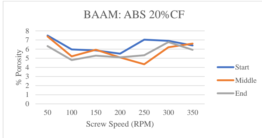
Figure 8. Porosity as a function of Screw Speed and Sample Location along the extruded bead
