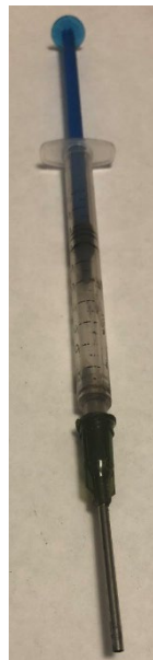
Figure 6 Needle like dropper used to measure solutions and binder
