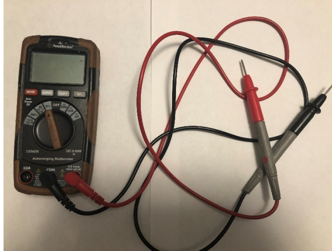
Figure 1 Auto-ranging multimeter conductivity measuring device
