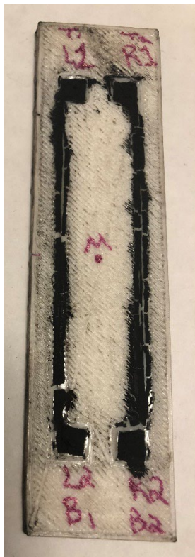
Figure 15 Example of experiment 1 copper tray cracks
