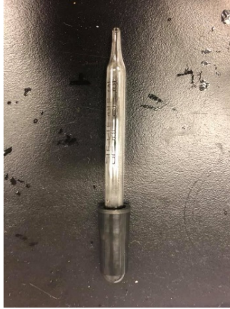
Figure 5 Initial dropper used to measure and inject 3D printed trays with NMP and nanoparticle solution
