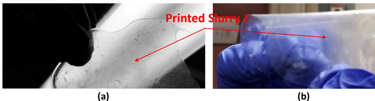
**Figure 7:** Properties of the air-dried Slurry J – (a) transparent and (b) flexible.
