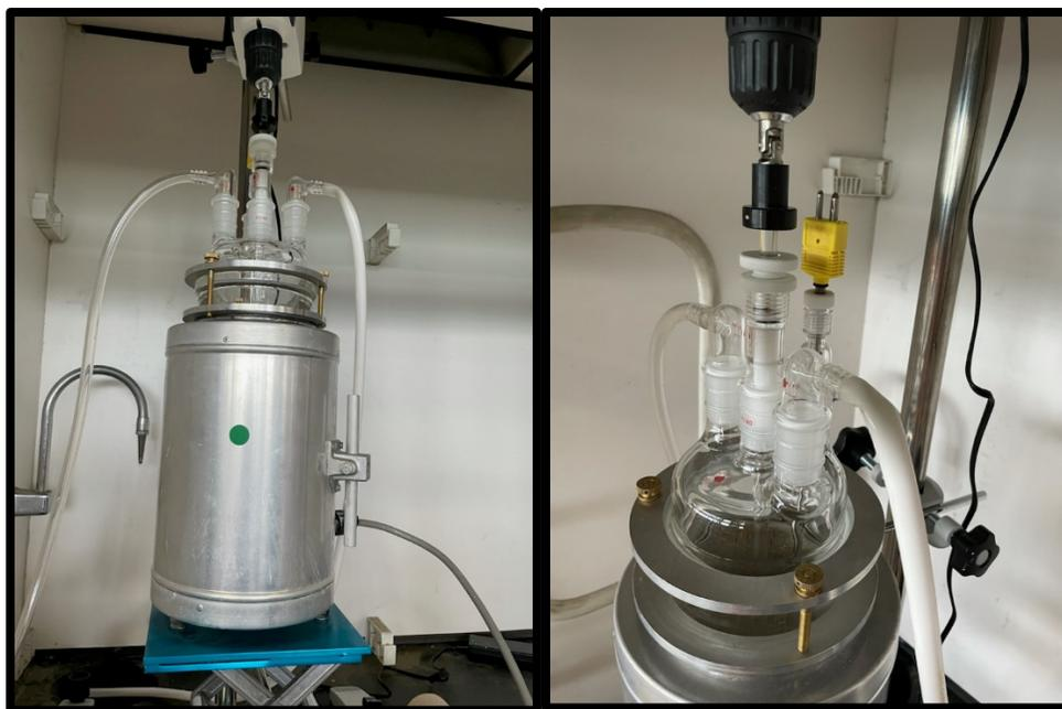
Figure 2: TIPS equipment overview (left) and close-up of fittings (right)
