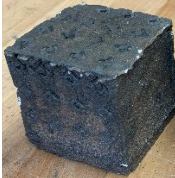
Figure 7: As-Cast 316L Stainless Steel Lattice Infiltrated with high Cr white iron
