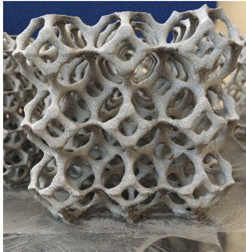
Figure 6: 316L Stainless Lattice Surface Finish
