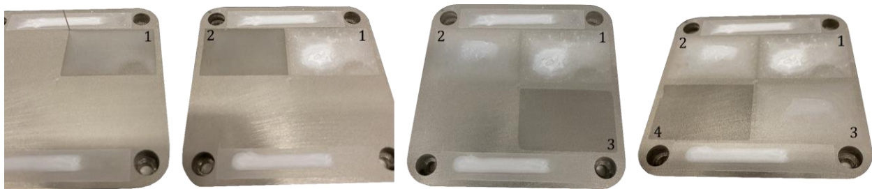
Figure 10 – Recently-deposited liquid alumina slurry diluted to different concentrations. Each image shows the deposition of a unique concentration to a different quadrant on the substrate. Left to right: 3 wt%, 2 wt%, 1 wt%, and 0.5 wt% slurry. Dopant agglomeration near the centers of the deposition areas is observed as more white (alumina) than the exterior regions of the depositions.
