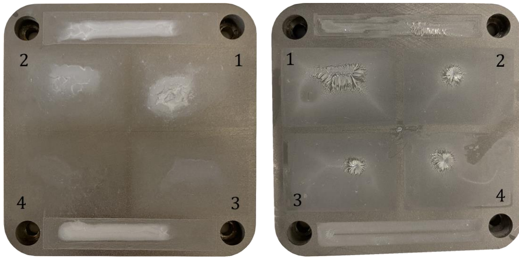
Figure 6 - Dried alumina (left) and zirconia (right) deposits performed using direct write deposition.
