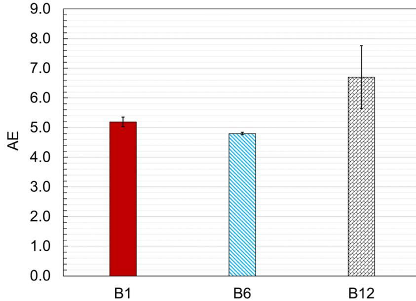
Fig. 6 AE values for IN718 powder in different reuse conditions. B1 implies virgin powder and B12 refers to the powder which was reused 11 times.
