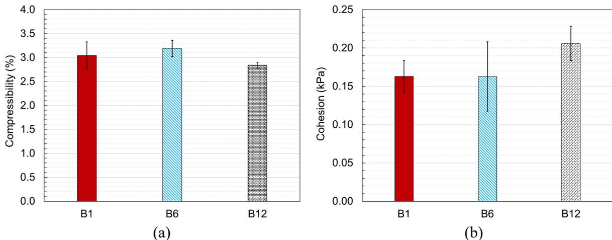
Fig. 3 IN718 powder rheological properties including (a) compressibility, and (b) cohesion for B1 (virgin powder), B6 (5x reused powder), and B12 (11x reused powder).
