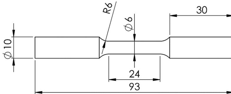
Fig. 2 The geometry of net-shaped tension test specimens according to ASTM E8. All dimensions are in mm.
