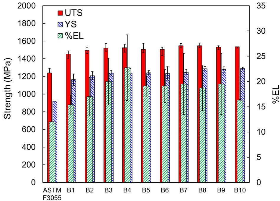
Fig. 5 Tensile properties including UTS, YS, and %EL for the LB-PBF IN718 specimens for different powder reuse iterations (B1-B10).
