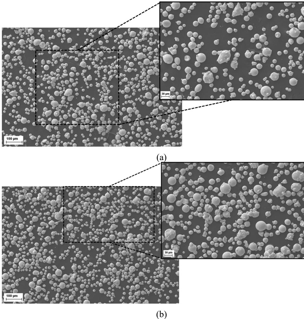
Fig. 4 Particle shape morphology for the (a) virgin (used for B1 fabrication) and (b) 9x reused powder (employed for B10 fabrication).
