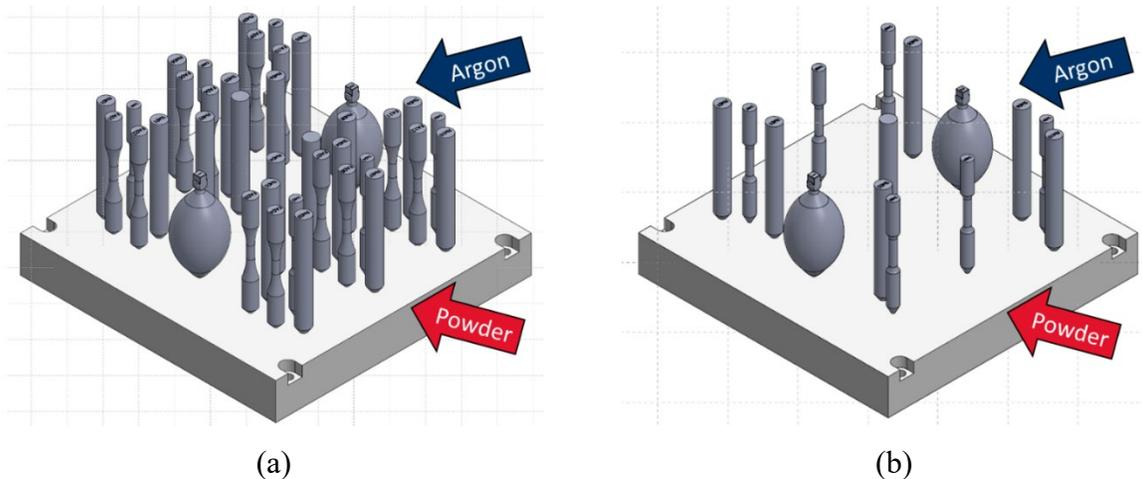
Fig. 1 (a) The full and (b) half build layouts including six net-shaped tension test specimens.
