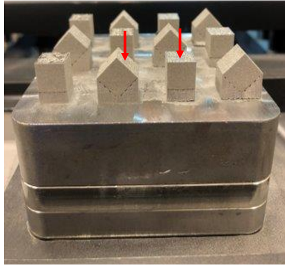
Figure 1: Vertically and diagonally built L-PBF Inconel 625 samples on build platform. Red arrows indicate the face used to measure microhardness.
