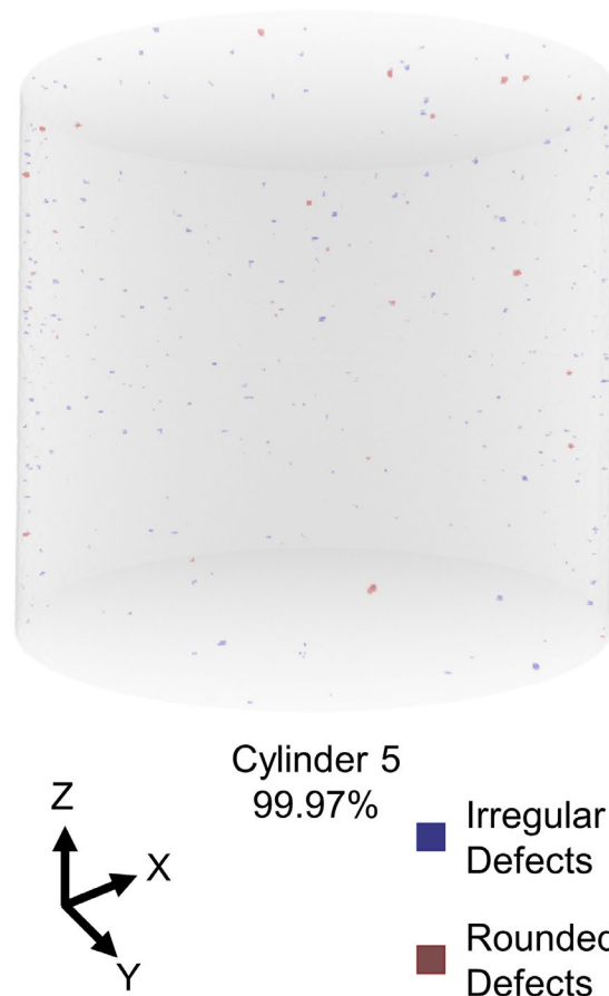
Figure 5. A three-dimensional visualization of the porous defect space (above 4 voxels) along the build direction (Z) from the XCT data of cylinder 5 (highest density), along with the density value obtained from the XCT data.
