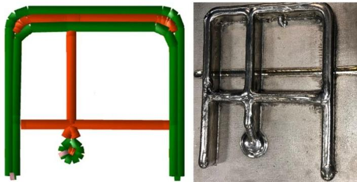
Figure 5: Example object constructed with automated profilometer support for height control. The system generated a height map after each layer construction. This height map was then used to adjust material flow for the subsequent layer. Left: Pathing from slicer. Right: Final
