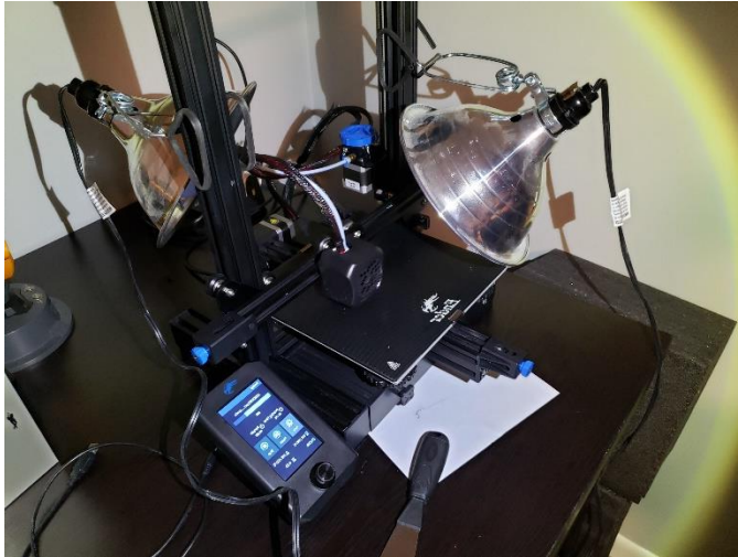
Figure 4. The test bed for the printing of the specimens. It consists of an Ender 3 V2 FDM printer and two 150 Watt heat lamps. The heat lamps have been placed to point directly at the center of the build plate at the same height and are 5 inches away from that point. By placing the heat lamps in opposing positions the part can be equally bathed in radiation.
