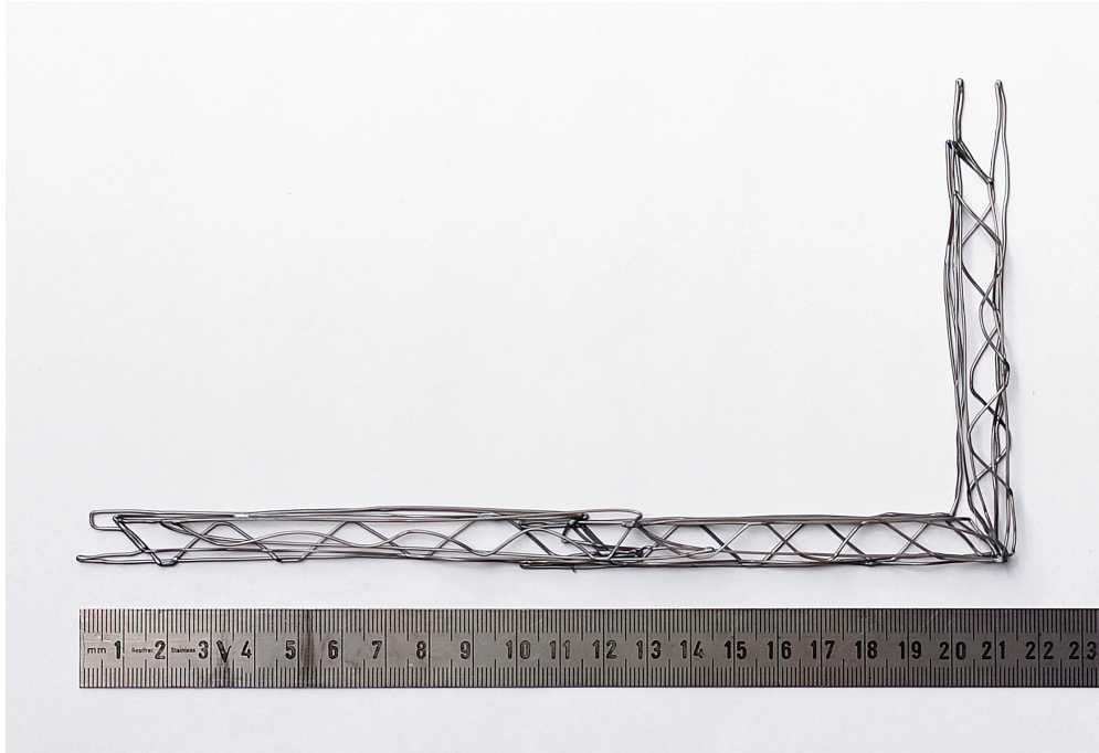
Fig. 9 'L' shaped truss for 2 dimensional structures with extension truss joined on 12 cm mark
