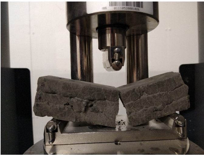
Figure 8: Failure under flexural strength test for specimen printed by piston based extruder (left) and auger screw based extruder system (on the right)
