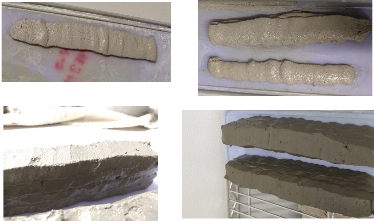
Figure 3: Illustration of 3D printed concrete with piston extruder using a variety of modified nozzles additively manufactured with fused filament-forming polylactic acid.
