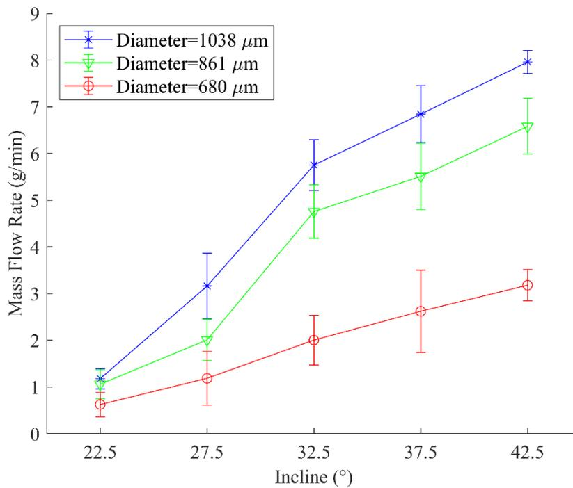
Figure 5: Mass flow rate versus nozzle incline angle results
