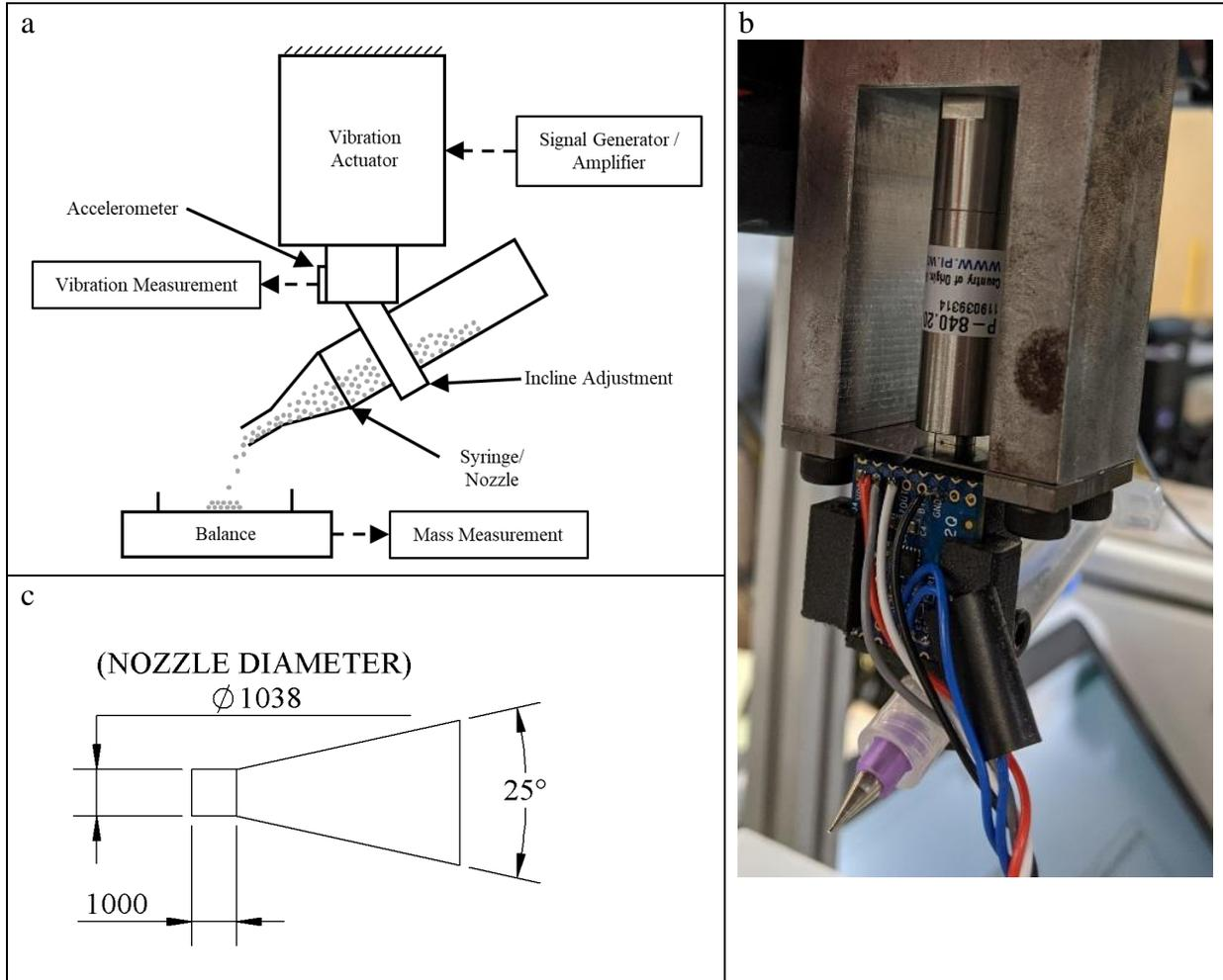
Figure 3: a) diagram of experimental setup b) picture of experimental setup c) inside dimensions of nozzle in microns
