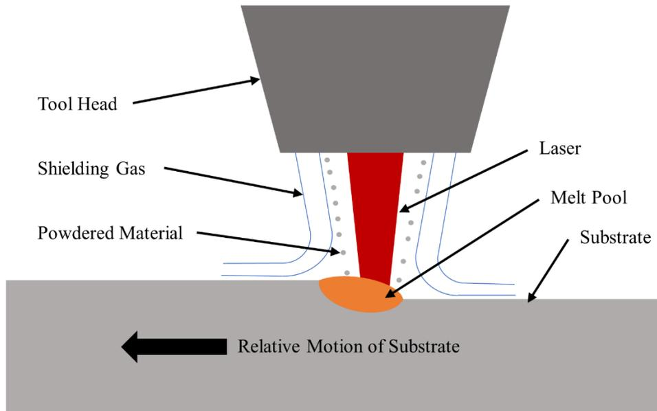
*Figure 1: Illustration of a typical blown-powder DED system*
