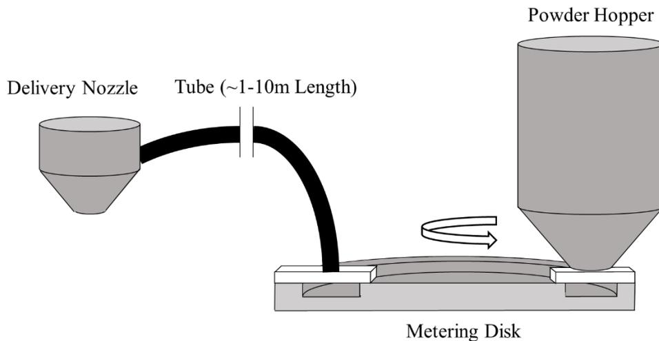
*Figure 2: An example conventional rotating disk powder delivery system*
