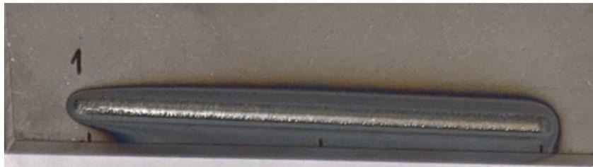
Figure 3: Clad created from first layer of experiment 1
