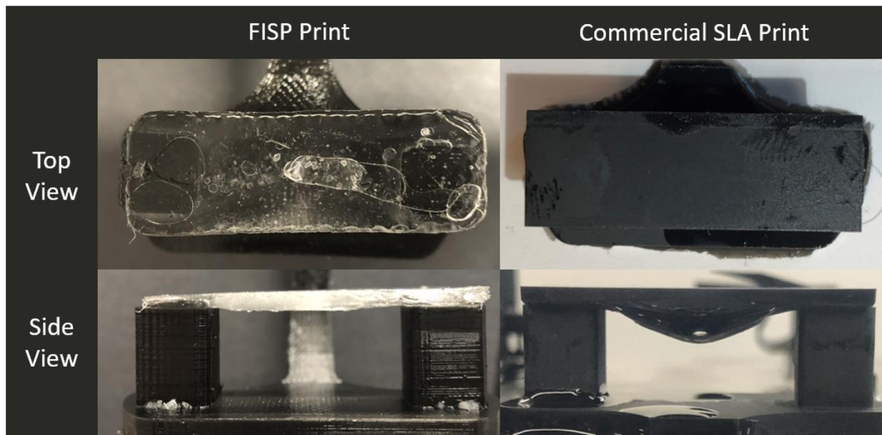
Figure 9: Unsupported bridge geometry comparison between a FISP print and a commercial SLA printer.
