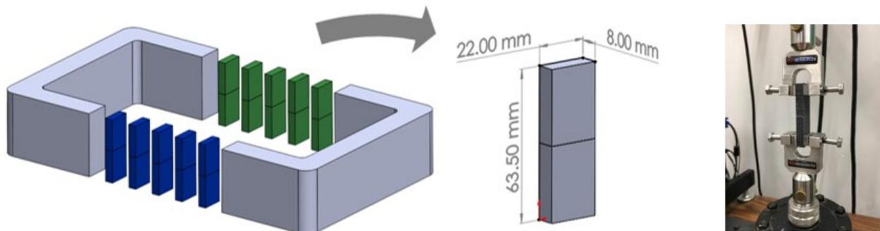
**Figure 4.** Tensile samples were cut from a four-sided object, with each side consisting of a unique sample set.
