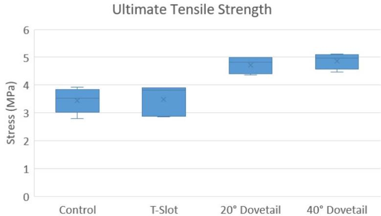
**Figure 7.** Ultimate tensile strength for each of the profiles.
