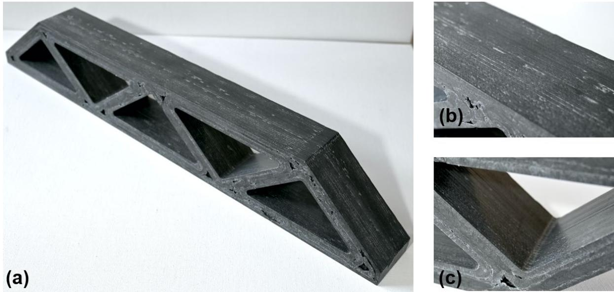
**Figure 9.** Images of the finished demonstration truss structure produced using iterative AM and subtractive manufacturing.
