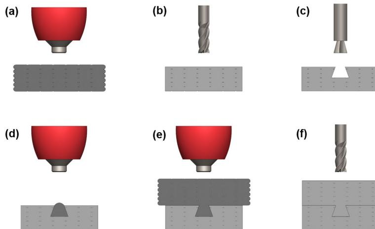
**Figure 2.** Proposed iterative process for hybrid additive and subtractive production of projects consists of a) AM deposition of a section of the object, b) cooling and machining, c) subtractive
