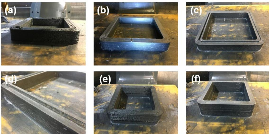
**Figure 5.** Demonstration of the proposed method of producing a mechanical interface to enable iterative AM and subtractive manufacturing consists of the process steps: a) AM deposition of a section of the object, b) subtractive machining of the surfaces, c) subtractive machining of grooves containing undercut geometry, d) AM filling of the grooves, e) deposition of another section of the object, f) final subtractive machining of the object.
