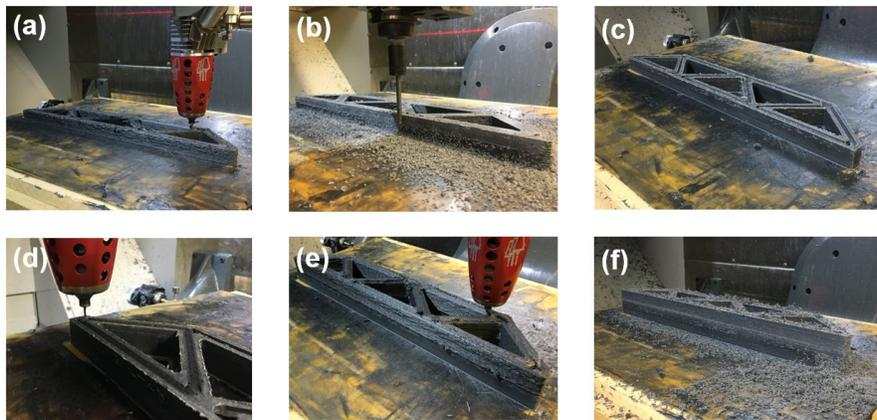
**Figure 8.** Demonstration truss structure produced by: a) AM deposition, b) machining, c) machining of 20° dovetail, d) AM dovetail filling, e) AM deposition, f) machining.
