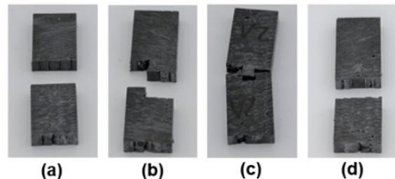
been shown to improve weld strength between layers [9]. Visual inspection of the T-slot samples showed incomplete groove filling, which may have reduced the mechanical interlocking that occurred on samples with that feature.
