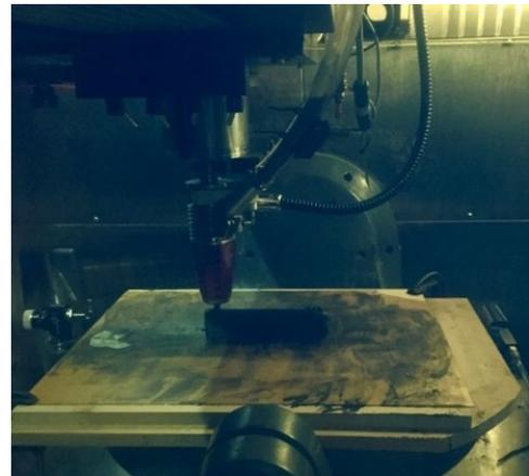
**Figure 1.** HAAS UMC750 machining center with a Hybrid Manufacturing Technologies AMBIT XTRUDE additive manufacturing system.
