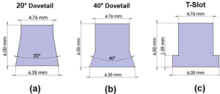
**Figure 3.** Profiles of undercut slots include a) 20° dovetail, b) 40° dovetail, and c) T-slot.
