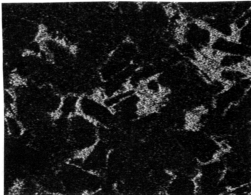
Fig 6c. Micrograph showing the distribution of the AlPO 4 phase as a coating around the alumina particles after heat treatment.
