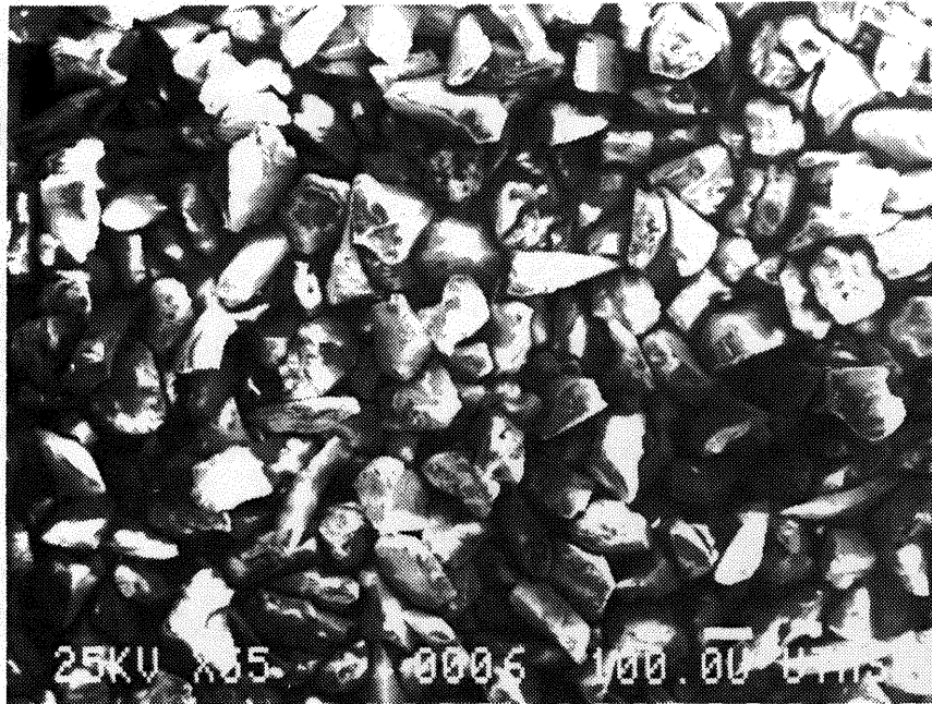
Fig 1. Micrograph of the as received Al 2 O 3 powder (< 150μm) showing the irregular shape of the particles.
