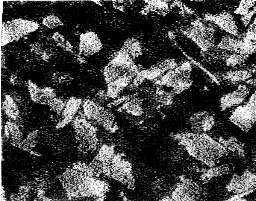
Fig6b. Micrograph showing the distribution of Al 2 O 3 phase in the area shown in Fig 6a
