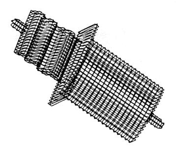
Figure 4: Robotic spray pathes
