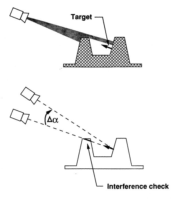
Figure 5: Interference checking
