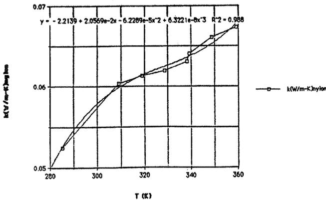
Figure 7. Thermal conductivities of nylon powder at different temperatures
