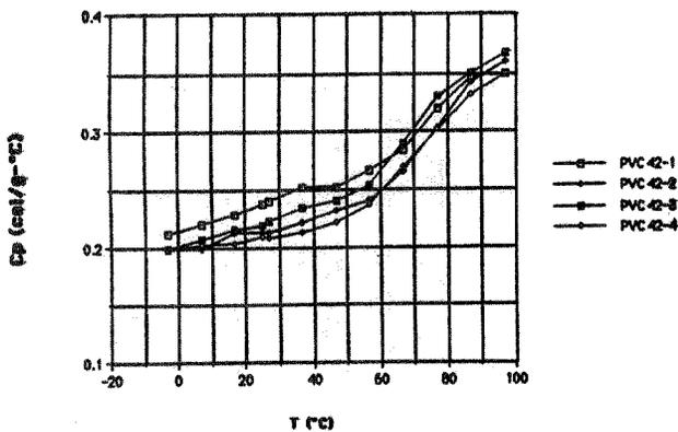
Figure 5. Cp (cal/g-°C) vs. temperature graph of four different kinds of PVC Powder
