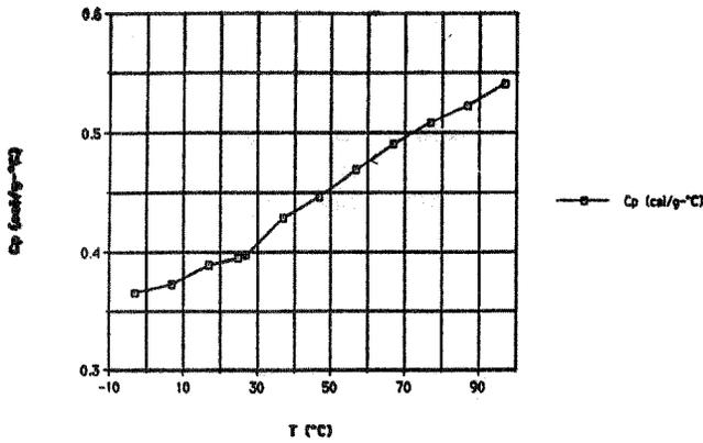
Figure 3. Cp (cal/g-°C) vs. temperature graph of nylon powder
