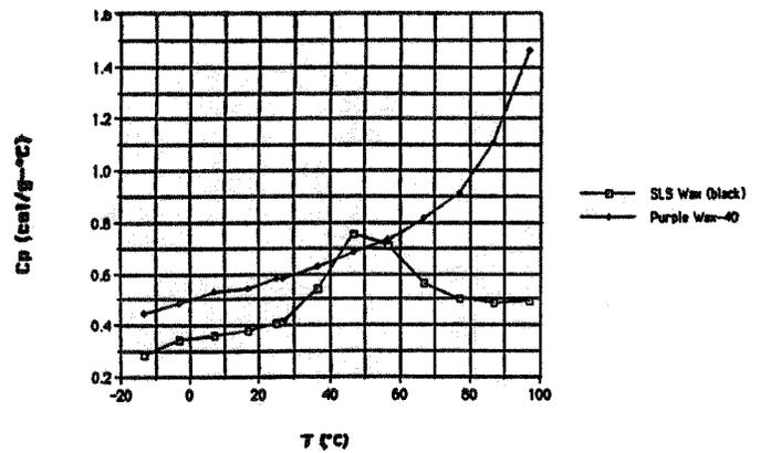
Figure 6. Cp (cal/g-°C) vs. temperature graph of Purple Wax-40 powder and SLS Wax (black) powders
