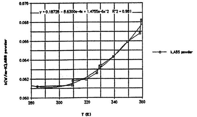
Figure 8. The thermal conductivities of ABS powder at different temperatures
