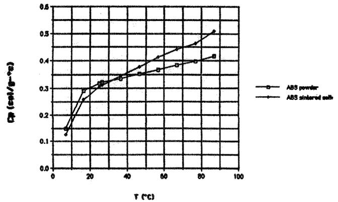
Figure 4. Cp (cal/g-°C) vs. temperature graph of ABS powder and the sintered solid obtained from ABS powder
