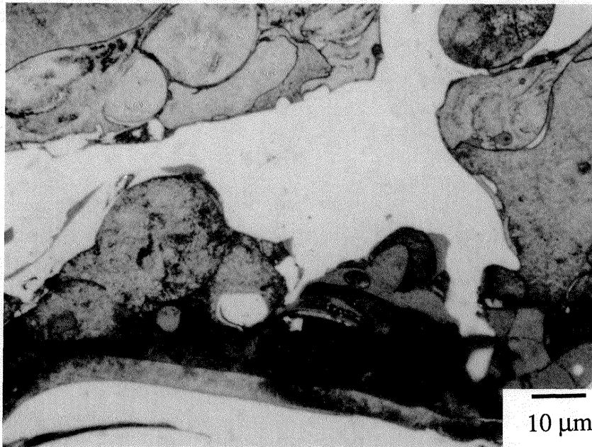
Fig. 15. Detail of inter-lamella region – pseudo-alloy of 0.8 % C steel and Invar.
