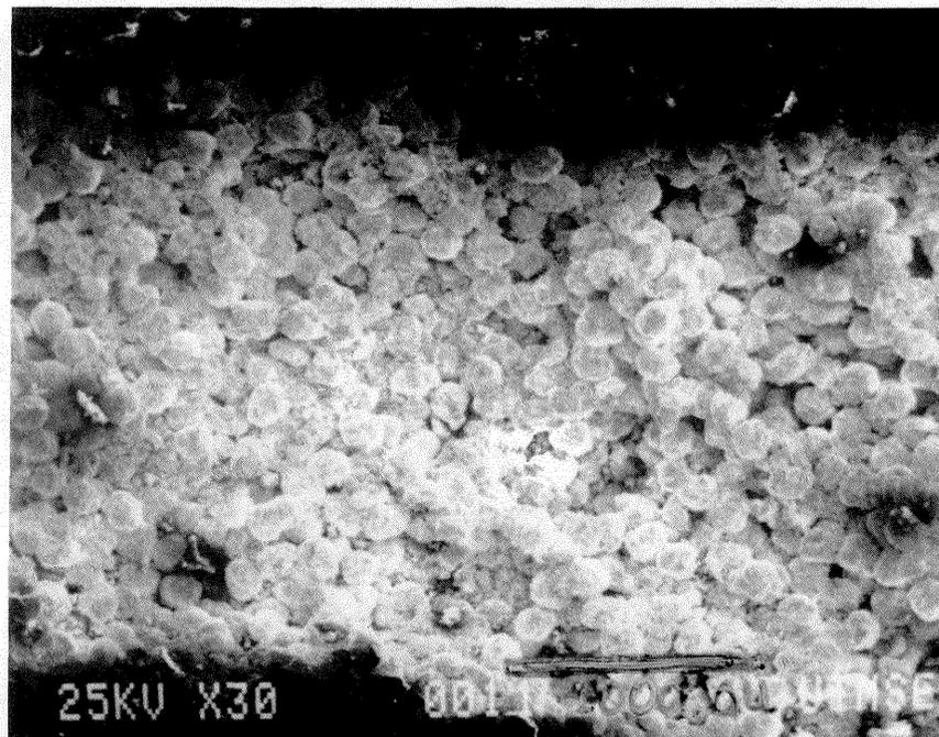
**Figure 7.** A cross section of an annealed sample (800°C for 24 hrs in H<sub>2</sub>). The layer are completely indistinguishable. The laser power was 17 W and the scan speed was 3.41 cm/s. The magnification is 30X.
