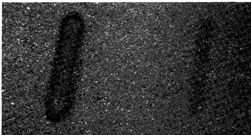
Figure 4: 3 mm line deposit on SiC. The line on the left was deposited from 500 Torr C_2H_2 precursor, and the line on the right was deposited from 500 Torr C_2H_2 /200 Torr CH_4 precursor.
