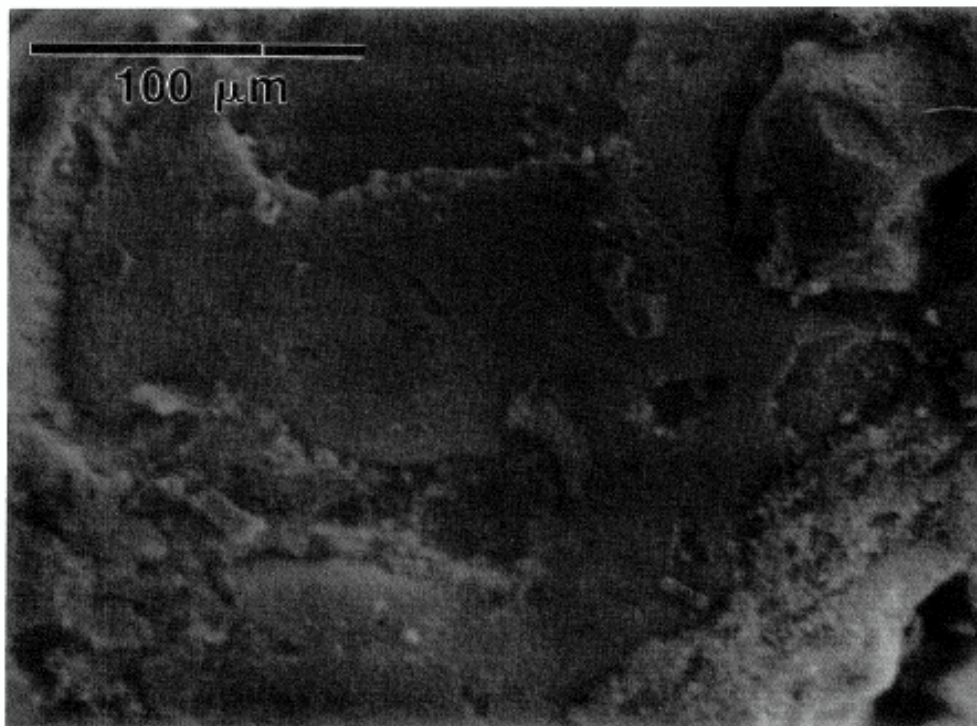
Figure 2. An enlarged view of an agglomerated region. It may be seen that these regions are very dense.
