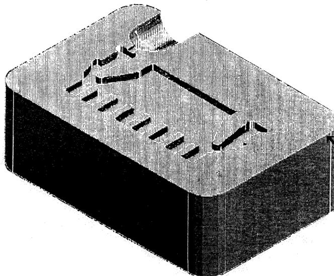
Figure 2. CAD Rendering of an Injection Molding Tooling Insert.
