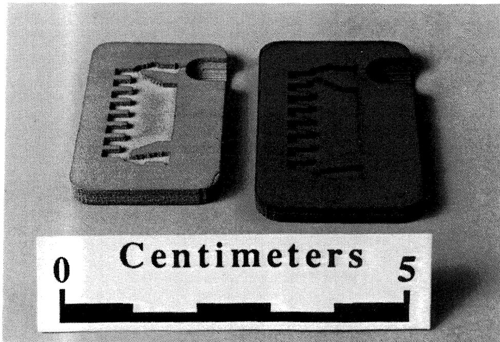
Figure 5. A 3D Printed Part Sintered to 78% Density (left) and a Green Part (right).
