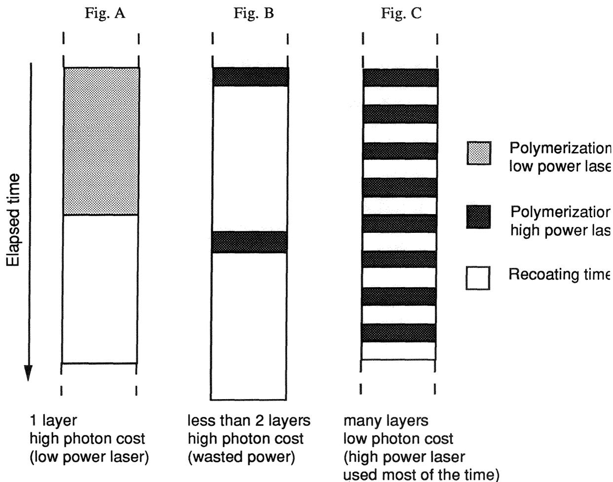
Fig. A shows that a small laser is properly dimensioned in the historical first generation SPL technology. One could therefore say that, given the current artificial constraints, first generation machinery is properly (not efficiently) defined.
