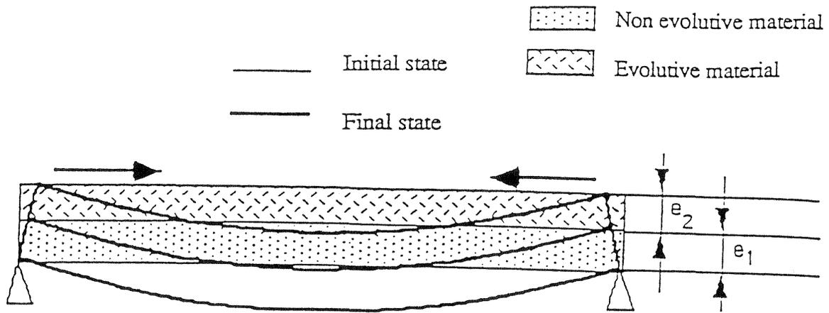
FIG. 3: Deformation induced by resin shrinkage (Simulation)
