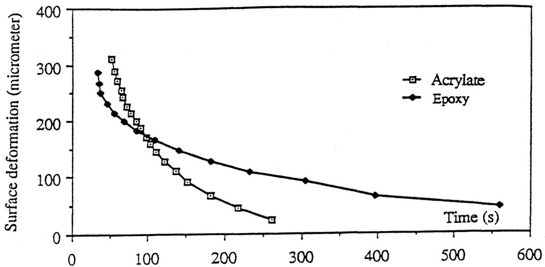
FIG. 2: Surface relaxation for two different resins
