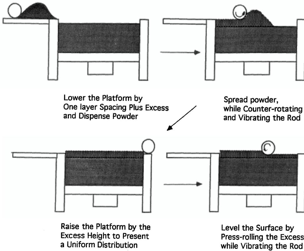
Figure 2. Press-rolling Sequence.
