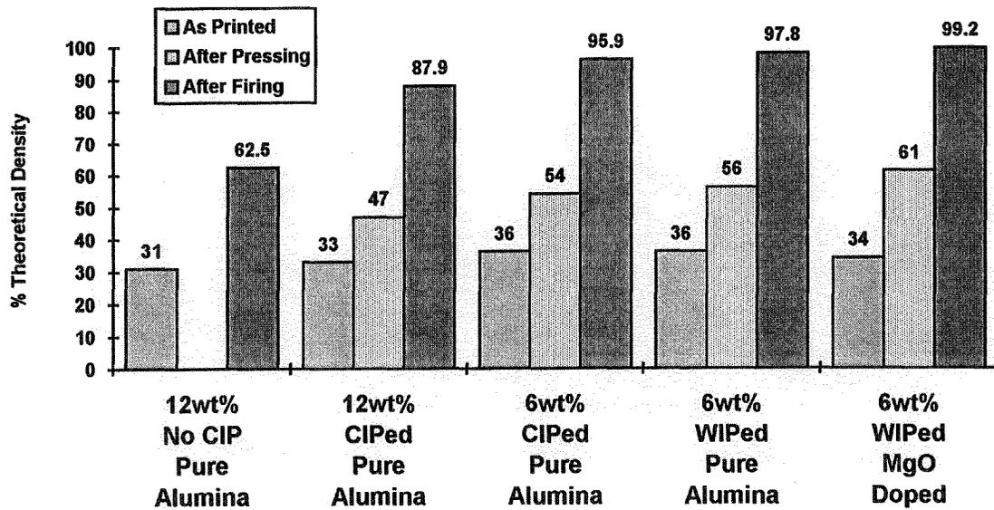
Figure 5. Bulk densities of parts at each stages.
