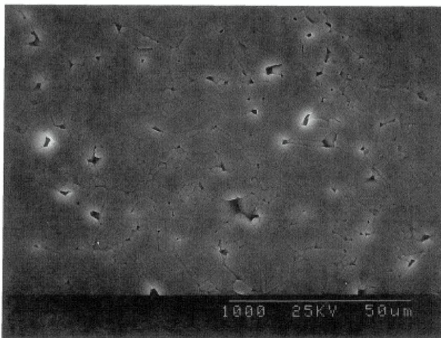
Figure 11. Thermally etched cross section ,MgO doped sample.(6wt% binder, WIPed)
