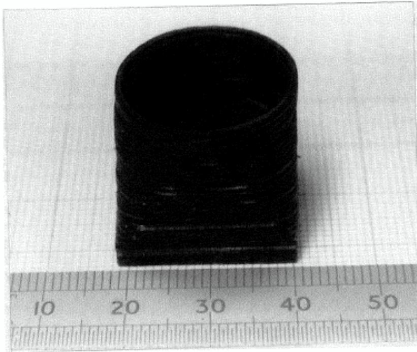
Figure 6. Square to circle transformation in 1mm thick stainless steel.
