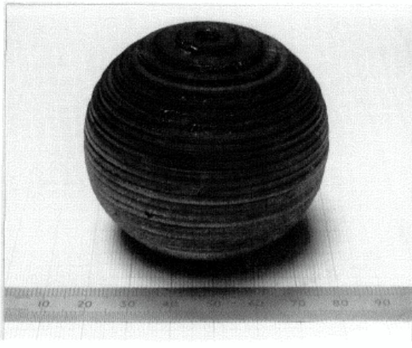
Figure 4. Sphere, produced in 2mm mild steel.
