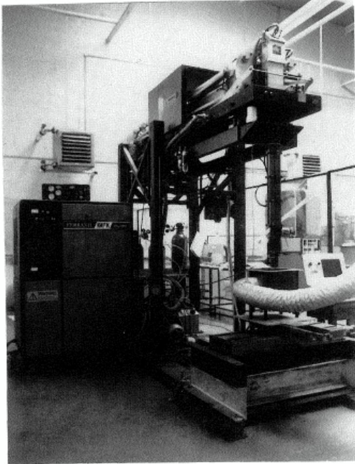
Figure 2. Ferranti MFK 1000 CO<sub>2</sub> laser
