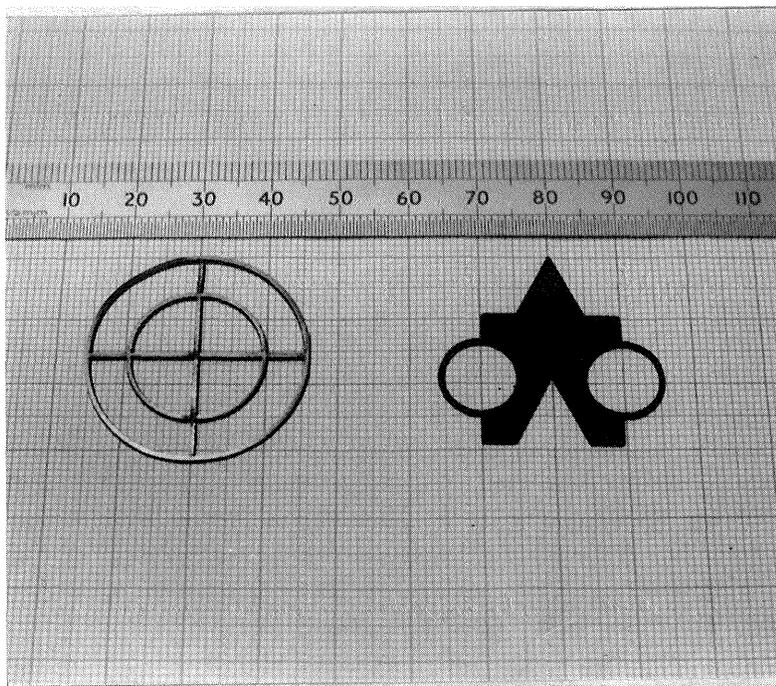
Figure 3. Laser cut parts in stainless steel
