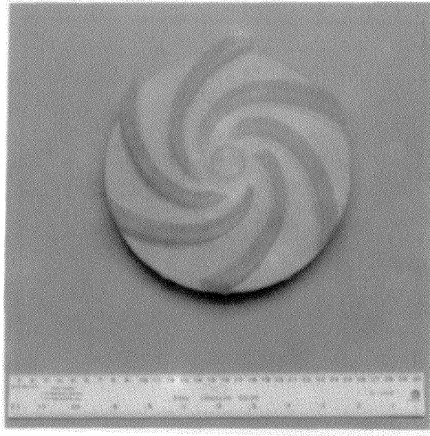
Figure 3. QuickCast™ SL pattern for the six-bladed centrifugal impeller.
