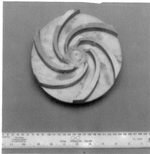
Figure 3. QuickCast™ SL pattern for the six-bladed centrifugal impeller.
