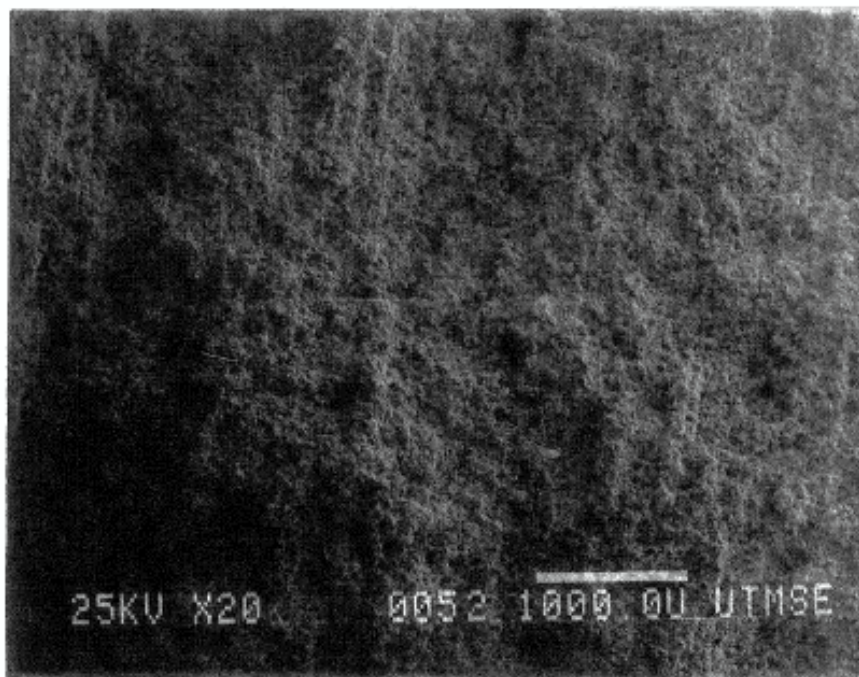
Figure 6. Good interlayer bonding. A_N = 2.00 \text{ cal/cm}^2 . Scanning conditions: 12W, 74 ips, and 3 mil beam spacing.
