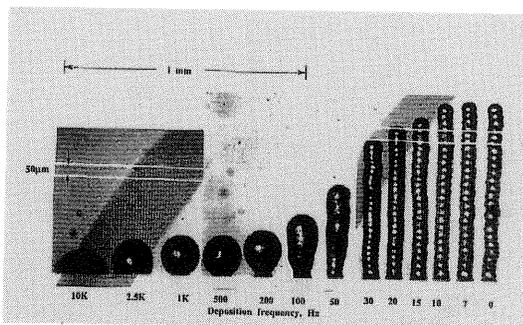
**Figure 3** Structures produced by depositing 25 microdrops on top of each other at various frequencies. Candelilla wax,  $T_0=100^\circ\text{C}$ ,  $T_a=38^\circ\text{C}$ .
