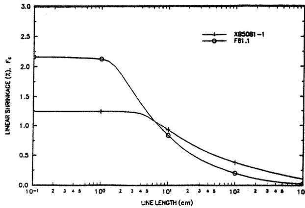
Shrinkage vs. length of line of plastic when
