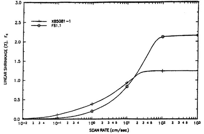
Shrinkage vs. scan rate for a 10 cm line of plastic.
