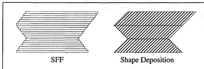
Figure 6: Comparison between SFF and Shape Deposition
