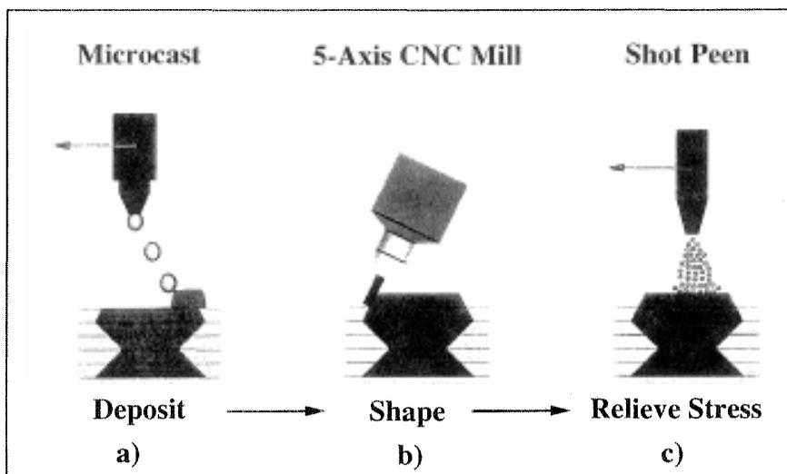
Figure 1: Creation of a layer using SDM
