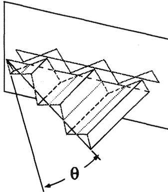
**Figure 2:** Approximation of a facet at an angle to the build direction
