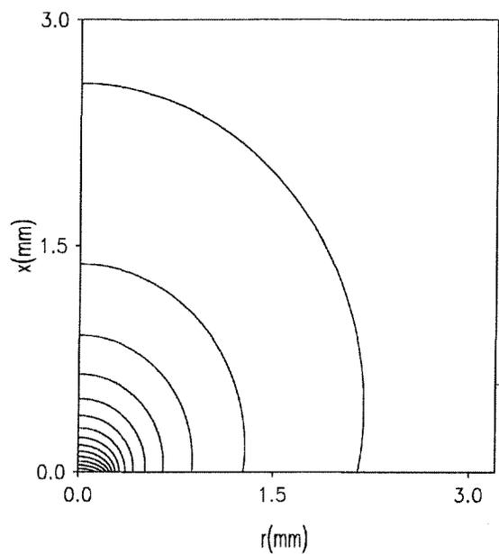
Fig. 4 Temperature distribution; from 1800 K to 400 K, step 100 K.
