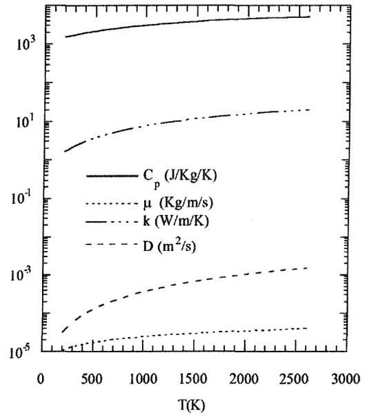
Fig. 2 Transport properties of TMS;  $D$  represents the binary diffusion coefficients of TMS in  $CH_4$  at 20 torr.
