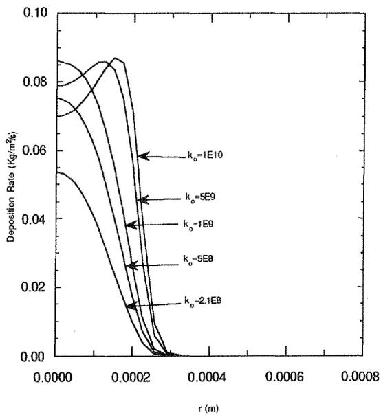
Fig. 7 Variation of deposition rate profiles with radial distance.
