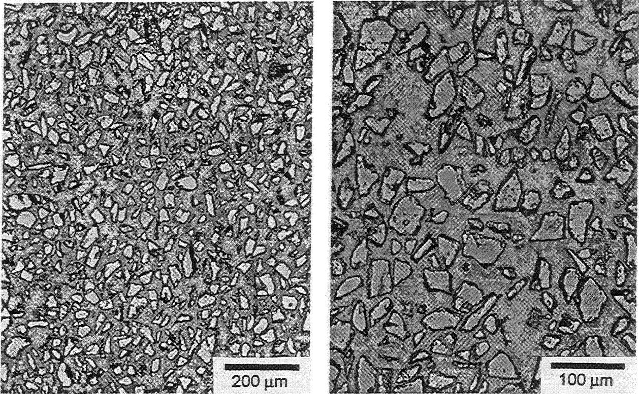
Figure 4. Micrographs of the infiltrated preforms. a)100X b)200X
