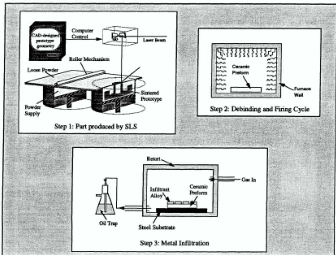
Figure 1. Schematic showing the three steps of the new production process.
