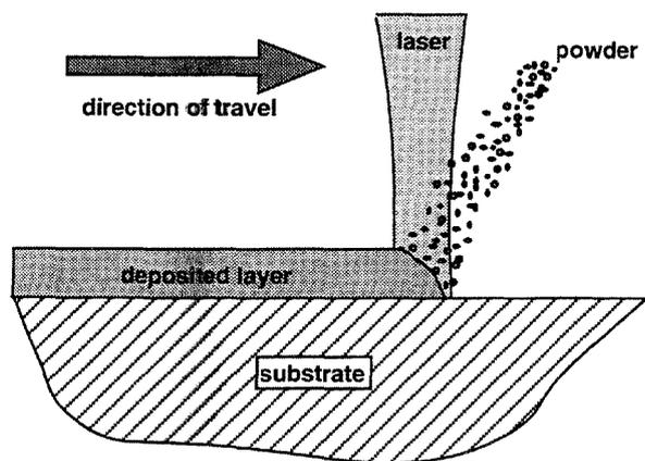
Figure 1: Schematic of laser deposition.
