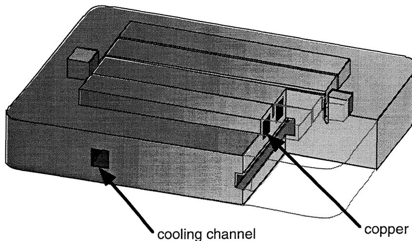
Figure 4: Schematic of half of injection molding tool with copper deposits.
