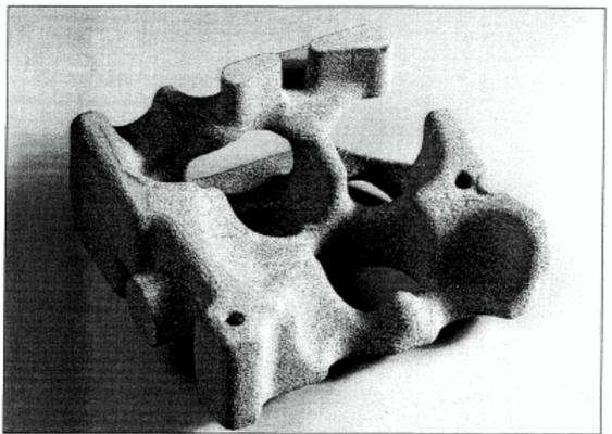
Fig 4: Core for the water cooling jacket of a 1-cylinder test engine
