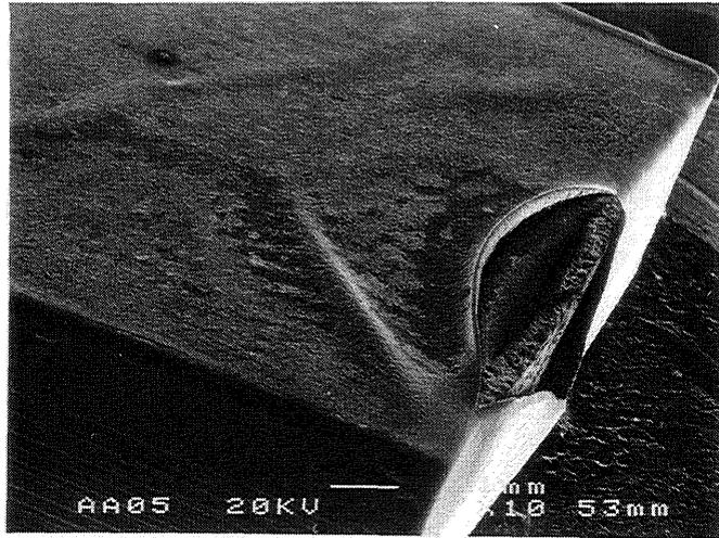
Figure 3 Electrode failure - Edge failure (15mm x 15mm SL 'tablet' electrode)
