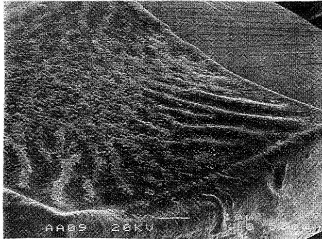
Figure 8 Electrode failure - Distortion (15mm x 15mm SL 'tablet' electrode)
