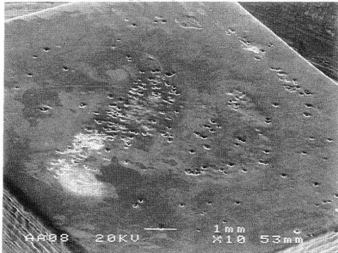
Figure 5 Porosity in electrodeposited copper, highlighted by pyrophosphate plating (15mm x 15mm SL 'tablet' electrode)
