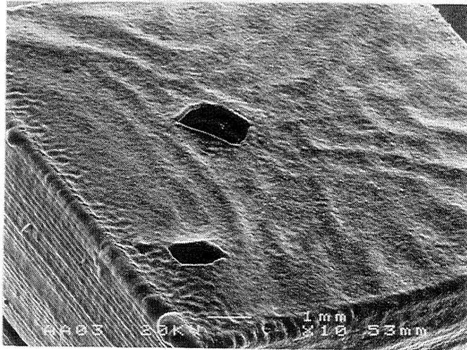
Figure 4 Electrode failure - Peppering (15mm x 15mm SL 'tablet' electrode)
