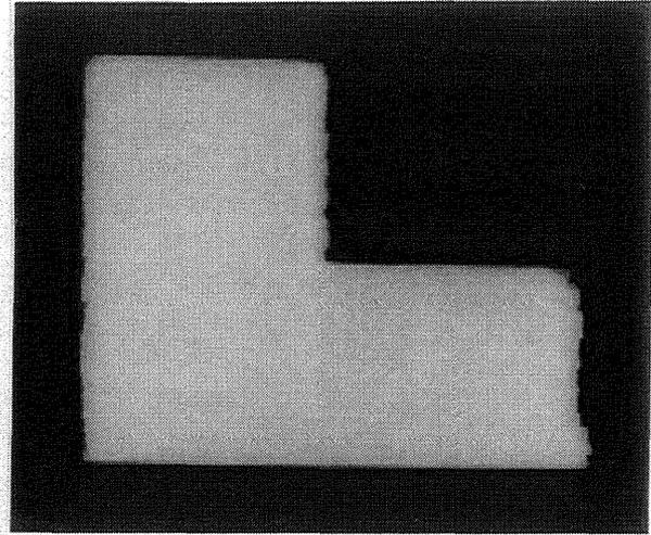
Figure 5. Optical micrograph of a sample laminated with fugitive-2, in which there was no delamination.
