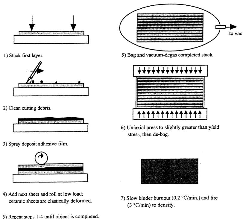
Figure 2. Schematic of the adhesive lamination process.
