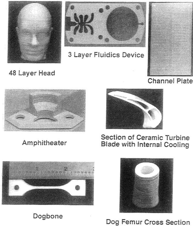
Figure 6. Catalog of ceramic CAM-LEM parts.
