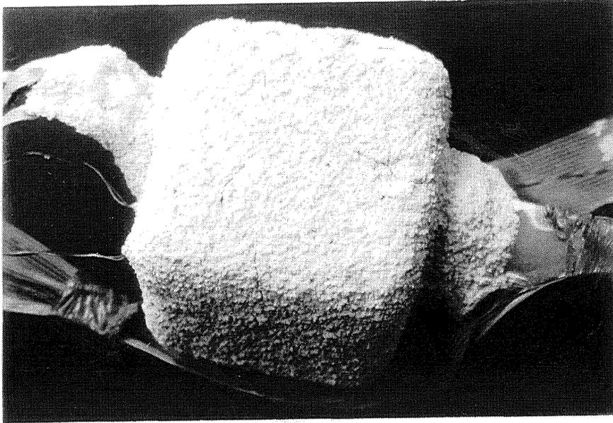
Note that the cracks propagate from the centre of each edge. This is consistent with the FEA work previously done.
