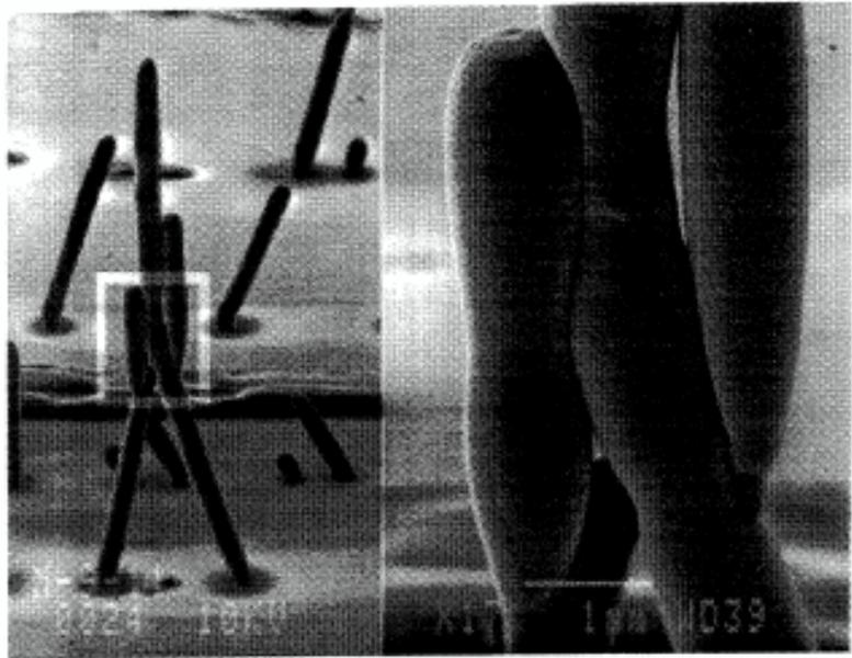
FIGURE 10. Sample 3-fiber braid atop a 1-level truss.
