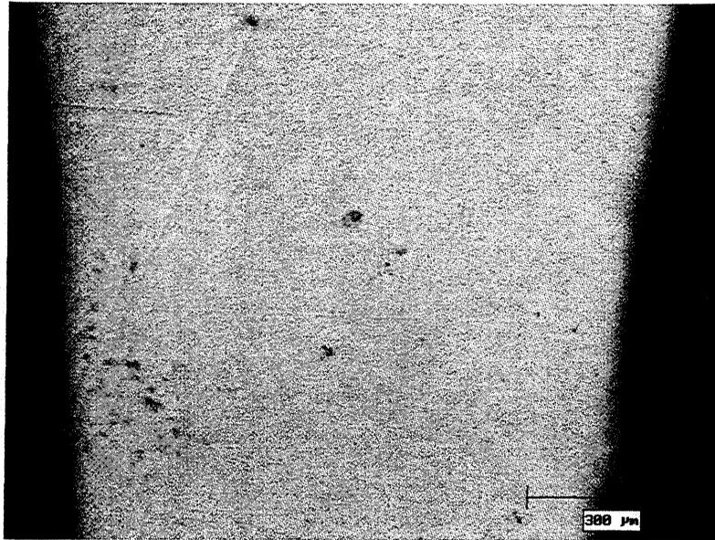
**Figure 8** PREP Ti-6Al-4V, single layer, as SLS processed
