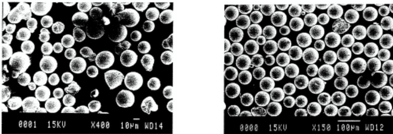
**Figure 2** SEM micrographs of -325 mesh Anval 625 (left) and -200 mesh PREP Ti-6Al-4V (right)
