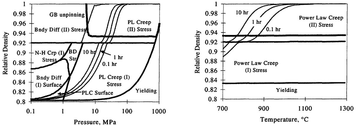
**Figure 7** Pressure HIP map (at 1240° C) for Inconel 625 (left) and temperature HIP map (at 165 MPa) for Inconel 625 (right)
